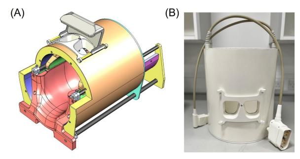
Figure 1. (A) 3D CAD model of the complete coil assembly and (B) Front view of the constructed coil with transmit and receive plugs.
