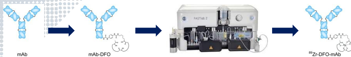
Figure 1: Schematic showing the aims of the project. Monoclonal antibodies (mAbs) are conjugated to DFO (DFO-NCS). mAb-DFO precursors undergo an automated radiolabelling procedure using the GE FASTLab platform. The outcome of this will be a ^{89}\text{Zr} radiolabelled radiopharmaceutical. Figure adapted from Zeglis and Lewis (2015).
