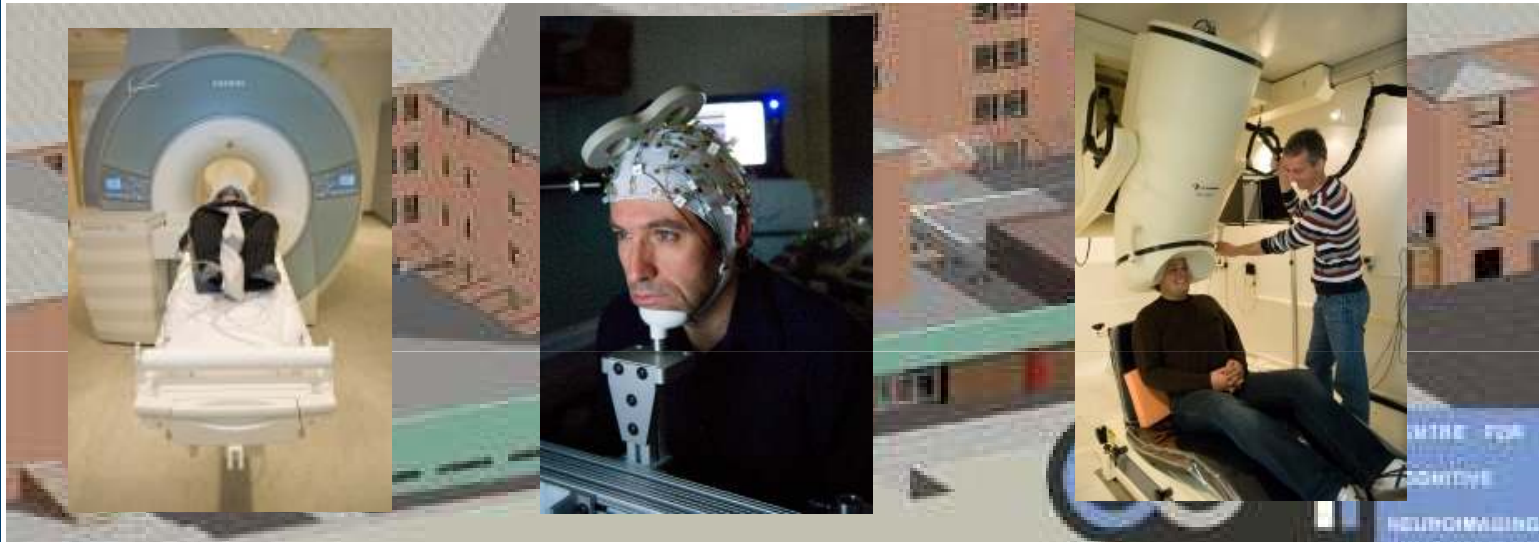
MEG – Biomag 4D 248-channel magnetometer
